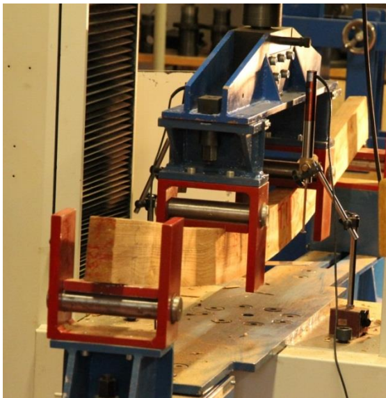
Figure 3.10 – Test piece from S. Miguel subject to static bending test
