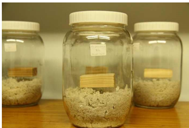
Figure 2.1 – Image from the start of test (EN 117:2005) using heartwood of sugi ( Cryptomeria japonica ).
