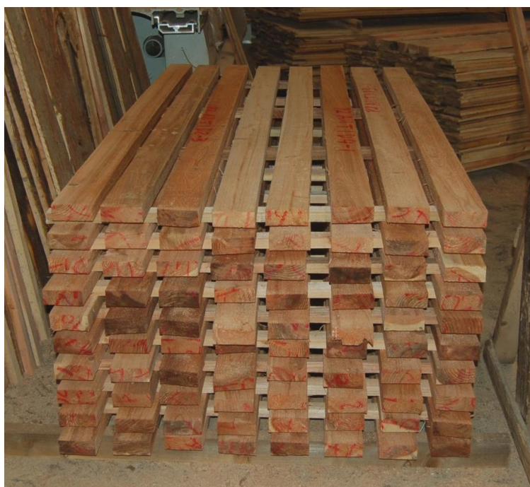
Figure 5. 80 test-pieces with dimensions 40mmx100mmx2000mm.
